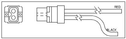
Figure 13 - Power Cable 19B802622P1 (USA Only)
